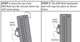
To remove UC-7410/7420-LX Plus from the DIN-Rail, simply reverse Steps 1 and 2 above.
